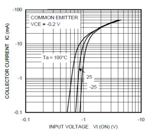
Fig. 10.2 RN2315 I<sub>C</sub>-V<sub>I(ON)</sub>
