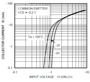
Fig. 10.3 RN2316 I<sub>C</sub>-V<sub>I(ON)</sub>
