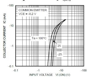
Fig. 10.5 RN2318 I<sub>C</sub>-V<sub>I(ON)</sub>
