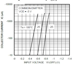
Fig. 10.6 RN2314 I<sub>C</sub>-V<sub>I(OFF)</sub>
