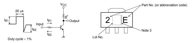
Figure 1 Switching Time Test Circuit & Timing Chart
