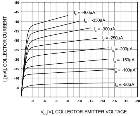
Figure 1. Static Characteristic
