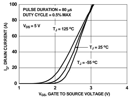
**Figure 5. Transfer Characteristics**
