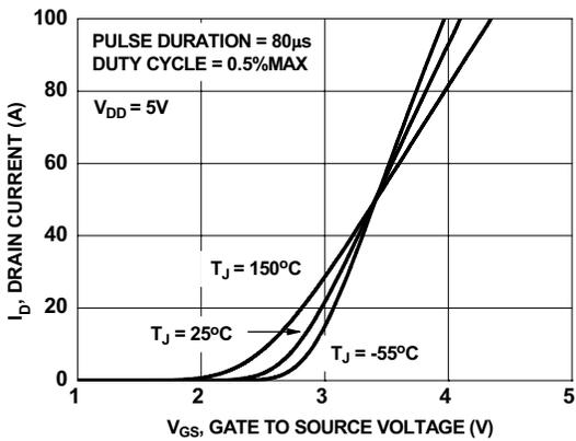
Figure 5. Transfer Characteristics
