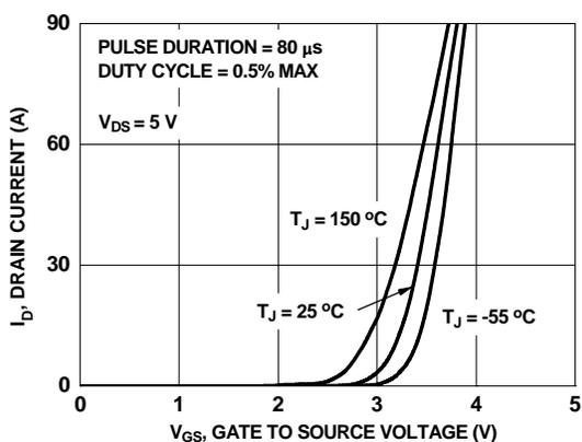
Figure 5. Transfer Characteristics
