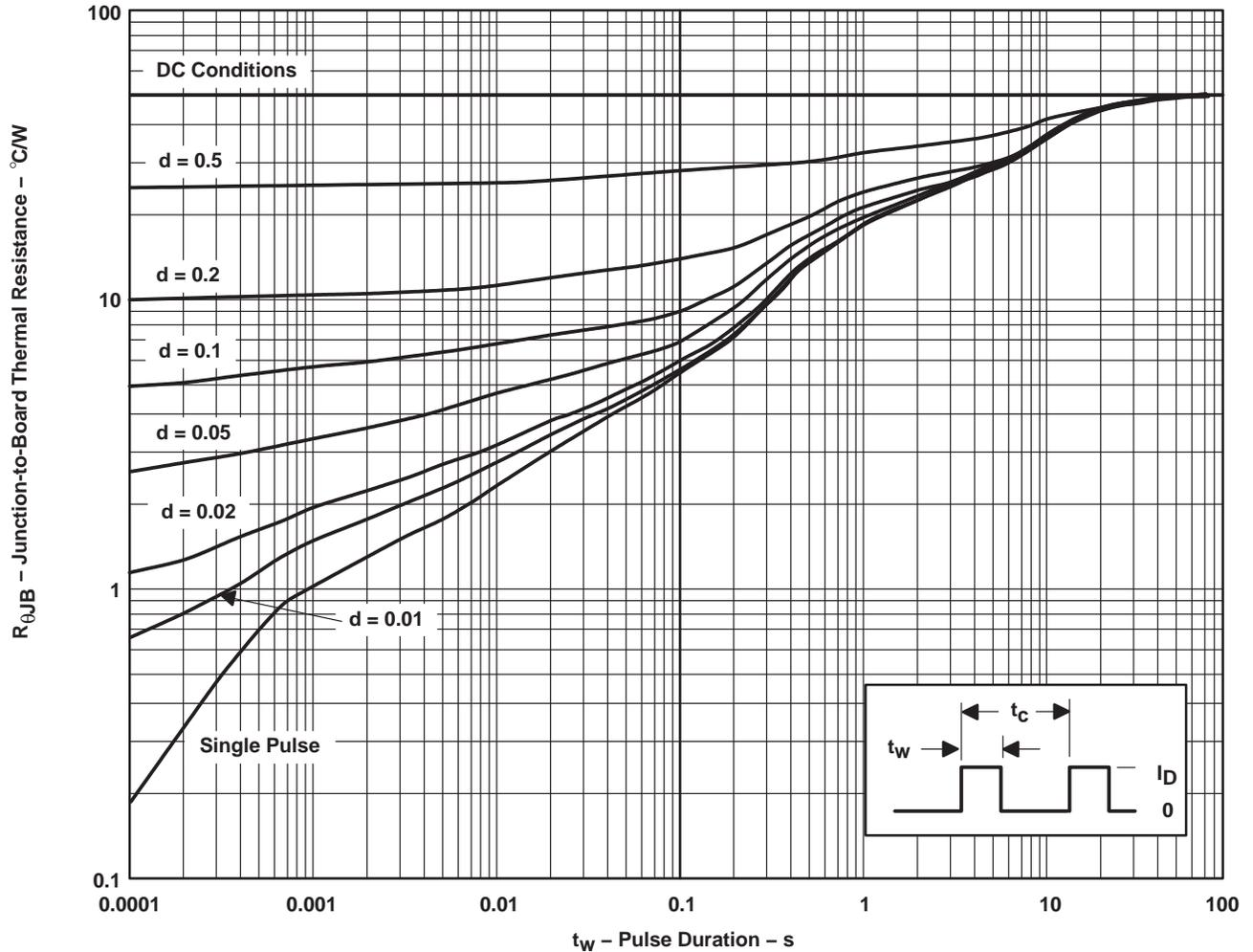
† Device mounted on 24in<sup>2</sup>, 4-layer FR4 printed-circuit board with no heatsink.
