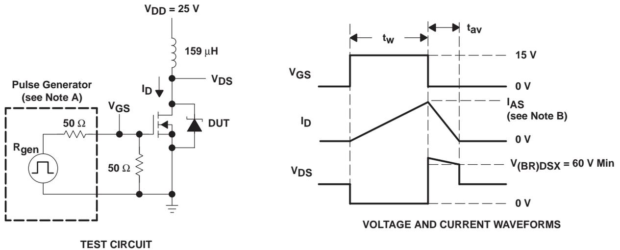
NOTES: A. The pulse generator has the following characteristics:  $t_r \leq 10$  ns,  $t_f \leq 10$  ns,  $Z_0 = 50 \Omega$ .
