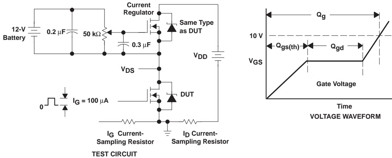
Figure 3. Gate-Charge Test Circuit and Voltage Waveform
