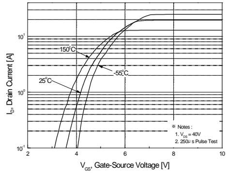
Figure 2. Transfer Characteristics
