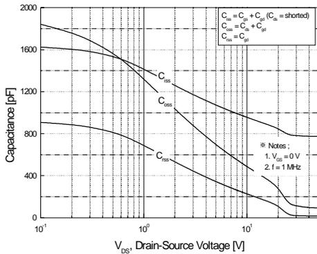
Figure 5. Capacitance Characteristics
