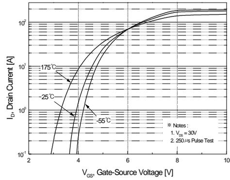
Figure 2. Transfer Characteristics
