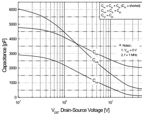
Figure 5. Capacitance Characteristics
