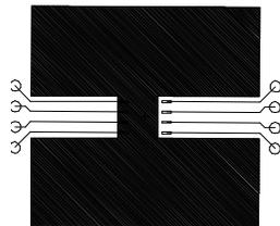
a.  $50^\circ\text{C/W}$  on a  $0.5\text{ in}^2$  pad of 2oz copper.
