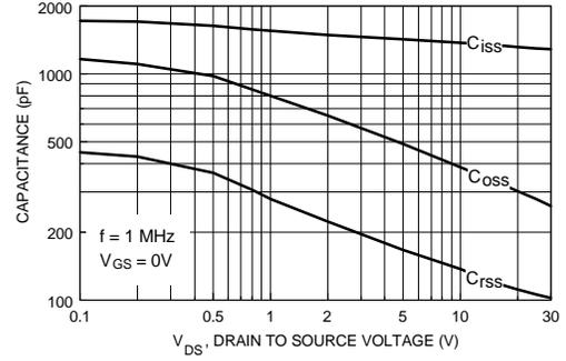
Figure 8. Capacitance Characteristics.
