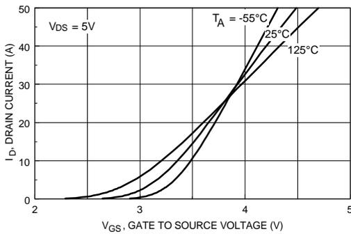
Figure 5. Transfer Characteristics.
