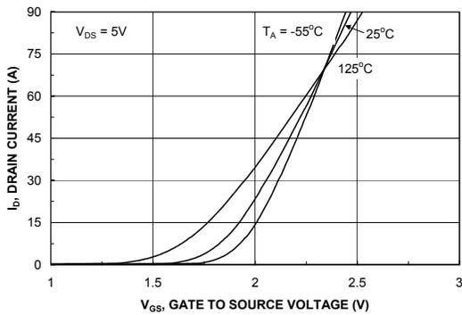
Figure 5. Transfer Characteristics.
