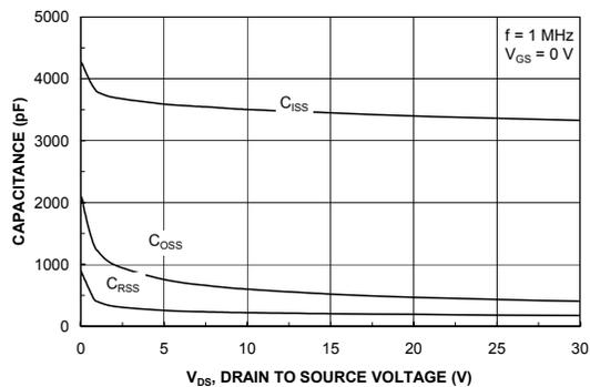
Figure 8. Capacitance Characteristics.
