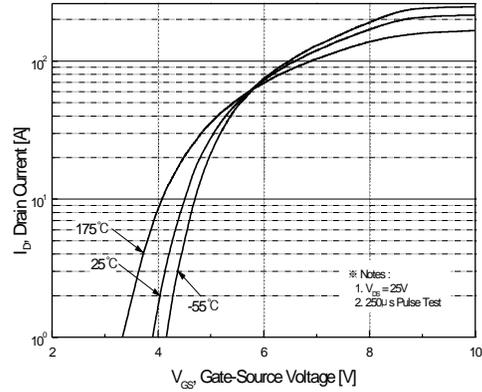
Figure 2. Transfer Characteristics
