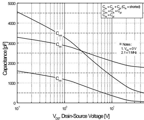
Figure 5. Capacitance Characteristics
