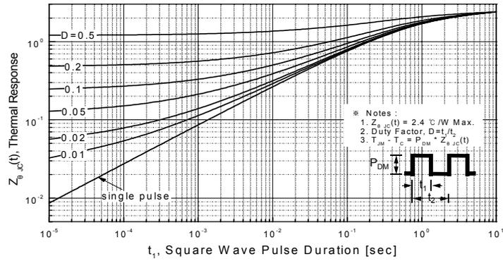
**Figure 11-2. Transient Thermal Response Curve for FQPF7N65C**
