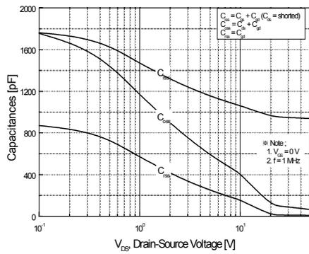
Figure 5. Capacitance Characteristics
