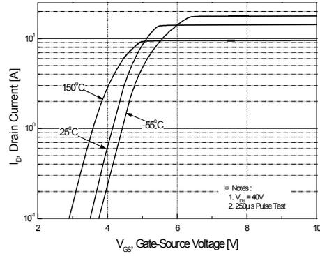
Figure 2. Transfer Characteristics
