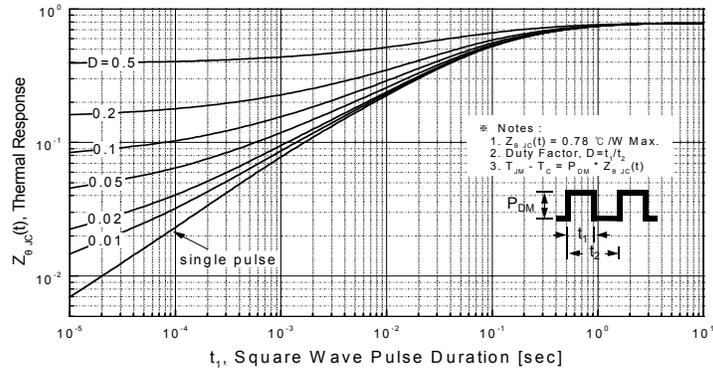
**Figure 11. Transient Thermal Response Curve for FQP7N65C**
