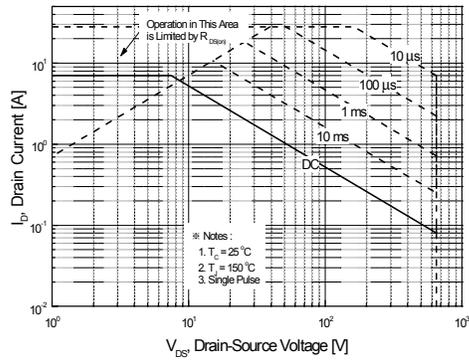
**Figure 9-2. Maximum Safe Operating Area for FQPF7N65C**
