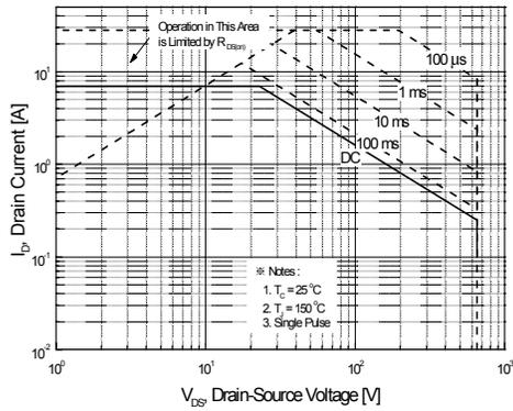
**Figure 9-1. Maximum Safe Operating Area for FQP7N65C**
