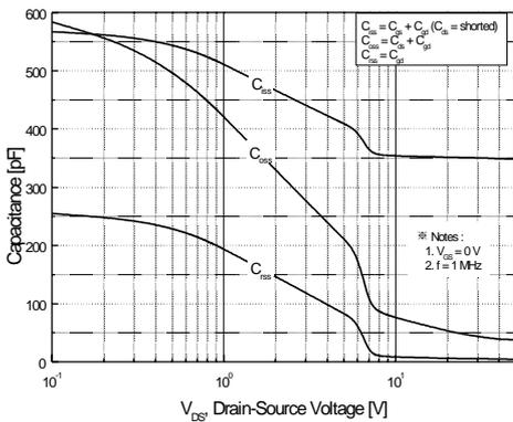
Figure 5. Capacitance Characteristics
