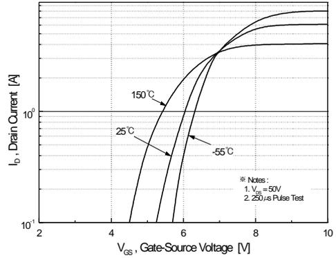
Figure 2. Transfer Characteristics
