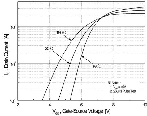
**Figure 2. Transfer Characteristics**
