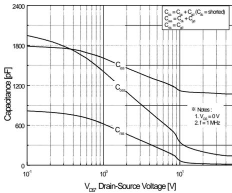
**Figure 5. Capacitance Characteristics**
