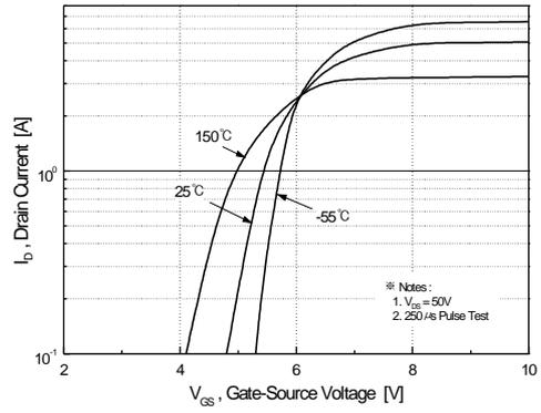
Figure 2. Transfer Characteristics
