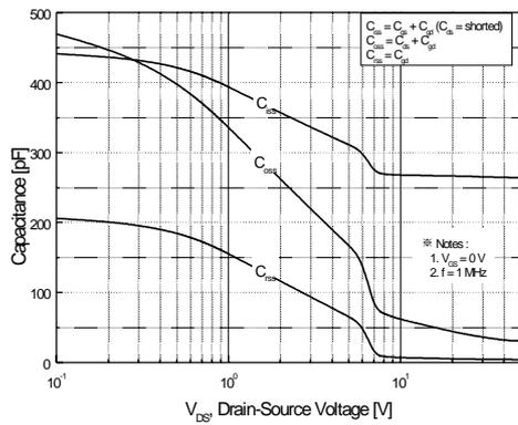
Figure 5. Capacitance Characteristics
