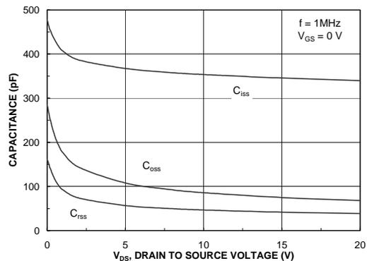
Figure 8. Capacitance Characteristics.
