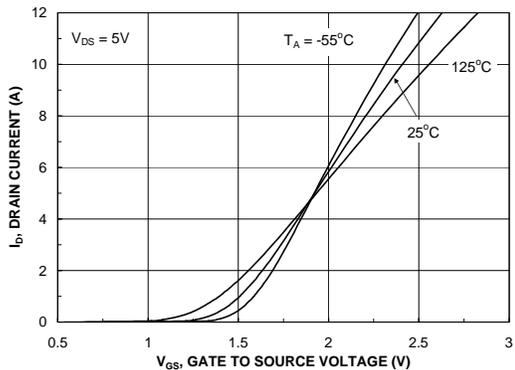
Figure 5. Transfer Characteristics.
