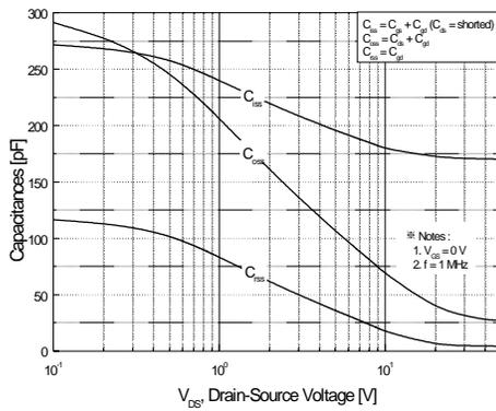
**Figure 5. Capacitance Characteristics**
