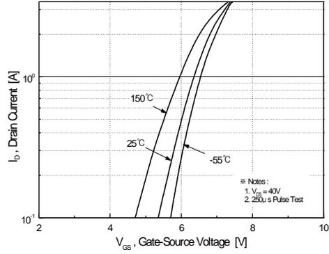
**Figure 2. Transfer Characteristics**
