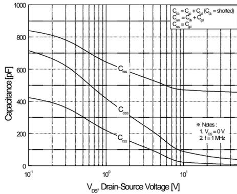
Figure 5. Capacitance Characteristics
