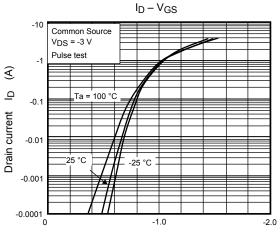
Gate-source voltage V<sub>GS</sub> (V)
