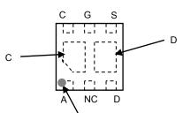
Polarity marking (on the top) \*Electrodes : on the bottom
