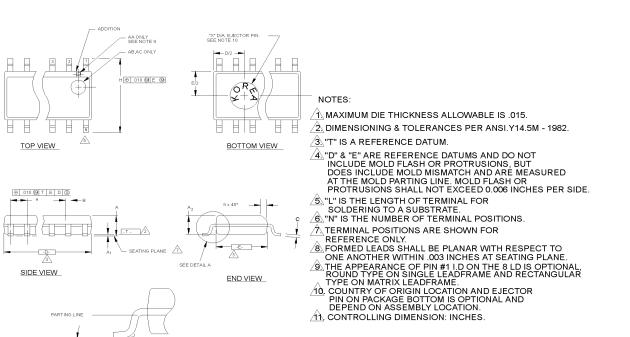
16-Pin Small Outlined Integrated Circuit (SOIC, 150-mil)
