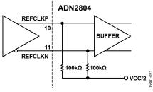
Figure 21. Differential REFCLK Configuration
