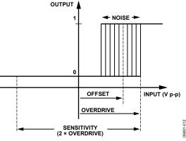
Figure 12. Input Sensitivity and Input Overdrive
