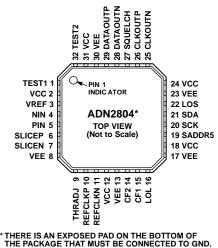
Figure 5. Pin Configuration
