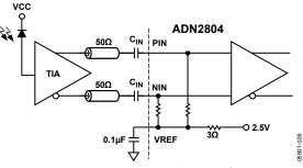
Figure 25. ADN2804 AC-Coupled Input Configuration
