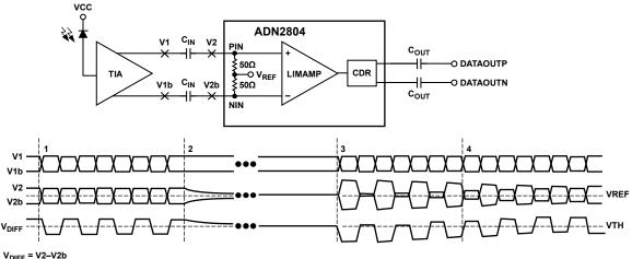
V<sub>DIFF</sub> = V2–V2b VTH = ADN2804 QUANTIZER THRESHOLD
