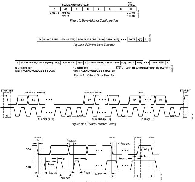
Figure 11. I<sup>2</sup>C Port Timing Diagram
