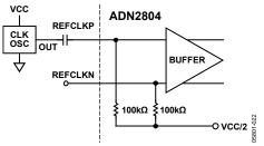
Figure 22. Single-Ended REFCLK Configuration
