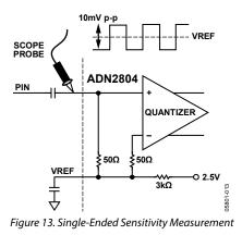
When the ADN2804 is driven differentially (see Figure 14), sensitivity seems to improve if observing the quantizer input with an oscilloscope probe. This is an illusion caused by the use of a single-ended probe. A 5 mV p-p signal appears to drive the ADN2804 quantizer; however, the single-ended probe measures only half the signal. The true quantizer input signal is twice this value, because the other quantizer input is a complementary signal to the signal being observed.
