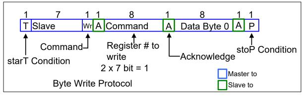
Figure 8. Byte Write Protocol
