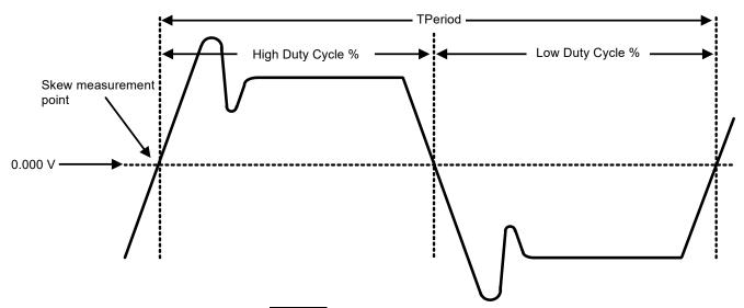
Figure 5. Differential (CLOCK–CLOCK) Measurement Points (T<sub>period</sub>, Duty Cycle, Jitter)
