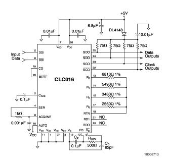
FIGURE 1. Typical +5V Connection - PLCC Package shown
