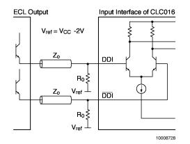
FIGURE 16. Differential 75Ω Source
