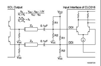
**FIGURE 17. AC Coupled Termination**
