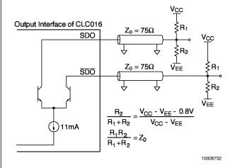
FIGURE 20. Load Terminated Output Interface
