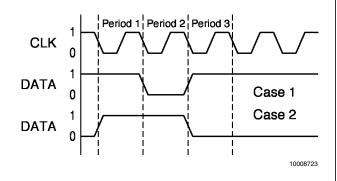
FIGURE 11. Harmonic Lock Detector Operation
