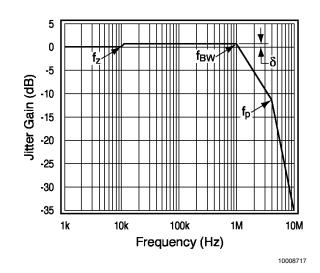
FIGURE 5. Closed-Loop Transfer Function
