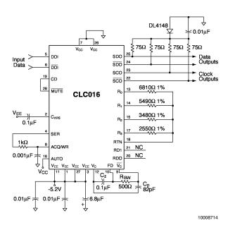
FIGURE 2. Typical –5.2V Connection - PLCC Package shown
