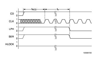
FIGURE 8. Data Rate Applied or Moves within PLL Capture
