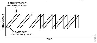
Figure 38. Delayed Start of Sawtooth Ramp
