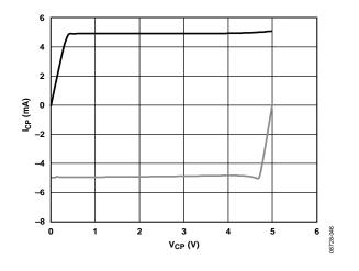
Figure 15. Charge Pump Output Characteristics
