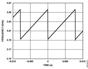
Figure 8. Sawtooth Waveform, PFD = 32 MHz, INT = 181, FRAC = 0, DEV Offset = 4, DEV Word = 20972, Step Word = 200, CLK<sub>2</sub> Divider = 10, CLK<sub>1</sub> Divider = 125
