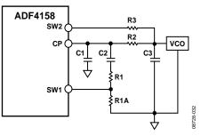
Figure 46. Fast-Lock Loop Filter Topology—Topology 1
