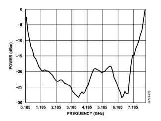
Figure 14. RF<sub>IN</sub> Sensitivity-Average Over Temperature and V<sub>DD</sub>
