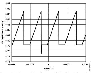
Figure 9. Delay Between Ramps for Sawtooth Waveform, PFD = 32 MHz, INT = 181, FRAC = 0, DEV Offset = 4, DEV Word = 20972, Step Word = 200, CLK<sub>2</sub> Divider = 10, CLK<sub>1</sub> Divider = 125, DEL Start Word = 1025
