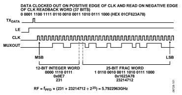
Figure 44. Reading Back Single Bits to Determine the Output Frequency at the Moment of Interrupt
