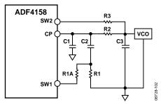
Figure 47. Fast-Lock Loop Filter Topology—Topology 2
