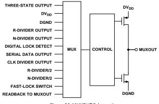
Figure 20. MUXOUT Schematic
