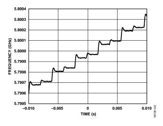
Figure 12. FSK Superimposed on Rising Edge of Triangular Waveform; Ramp Settings: PFD = 32 MHz, INT = 181, FRAC = 0, DEV Offset = 4, DEV Word = 20972, Step Word = 200, CLK DIV = 10, CLK<sub>1</sub> Divider = 125; FSK Settings: DEV Offset = 3, DEV Word = 4194
