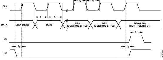
Figure 2. Write Timing Diagram
