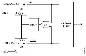
Figure 19. PFD Simplified Schematic
