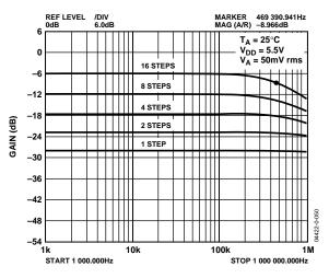
Figure 22. Gain vs. Frequency vs. Code,  $R_{AB} = 10 \text{ k}\Omega$
