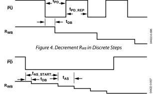
Figure 5. Decrement R<sub>WB</sub> in Autoscan Mode
