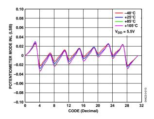
Figure 12. INL vs. Code,  $V_{DD} = 5 V$
