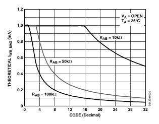
Figure 29. Maximum I<sub>WB</sub> vs. Code
