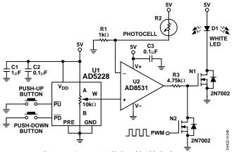
Figure 44. Automatic LCD Panel Backlight Control
