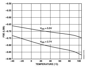
Figure 15. Full-Scale Error vs. Temperature
