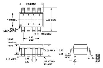
\*COMPLIANT TO JEDEC STANDARDS MO-193-BA WITH THE EXCEPTION OF PACKAGE HEIGHT AND THICKNESS. Figure 48. 8-Lead Small Outline Transistor Package [TSOT] (UJ-8)
