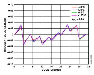
Figure 8. R-INL vs. Code vs. Temperature,  $V_{DD} = 5 V$
