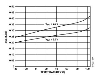
Figure 16. Zero-Scale Error vs. Temperature
