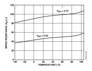
Figure 19. Wiper Resistance vs. Temperature
