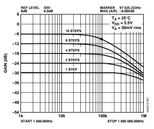
Figure 23. Gain vs. Frequency vs. Code,  $R_{AB} = 50 \text{ k}\Omega$
