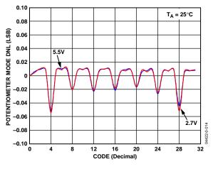
Figure 13. DNL vs. Code vs. Supply Voltages
