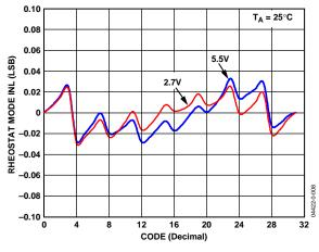
Figure 7. R-INL vs. Code vs. Supply Voltages
