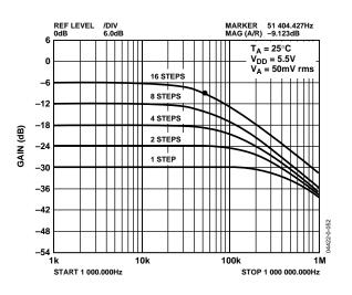
Figure 24. Gain vs. Frequency vs. Code,  $R_{AB} = 100 \text{ k}\Omega$
