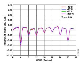
Figure 10. R-DNL vs. Code vs. Temperature,  $V_{DD} = 5 V$
