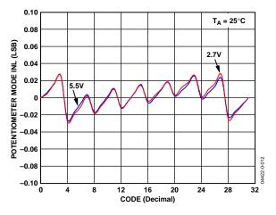
Figure 11. INL vs. Code vs. Supply Voltages
