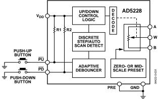
Figure 30. Typical Pushbutton Interface
