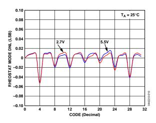
Figure 9. R-DNL vs. Code vs. Supply Voltages
