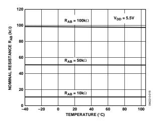
Figure 18. Nominal Resistance vs. Temperature
