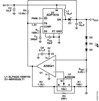
Figure 43. Adjustable Current Source for LEDs in Series
