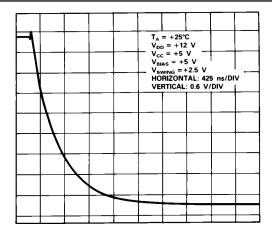
Figure 10. Negative-Going Settling Time
