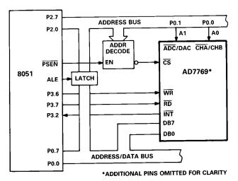
Figure 20. AD7769 to 8051 (Processor Bus) Interface
