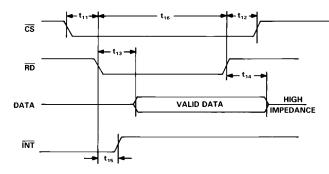
Figure 12. Timing for ADC Data Read
