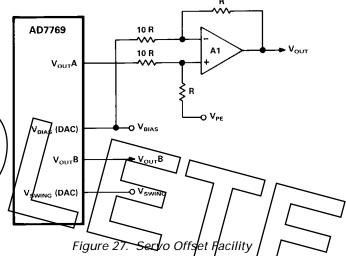
With no offset added,  $V_{OUT} = V_{PE}$ , where  $V_{PE}$  is the position error voltage which the servo loop normally drives to its zero level,  $V_{BIAS}$ . When an offset voltage is supplied by DAC A, the action of the servo is to move the head away from its current on-track position until the position error voltage is equal and opposite to the offset voltage. The position of the head about the track centre is thus programmable.
