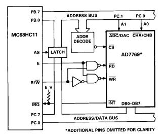
Figure 22. AD7769 to MC68HC11 Interfaced
