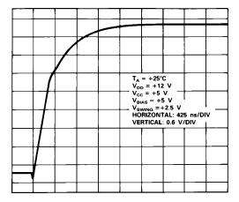
Figure 9. Positive-Going Settling Time
