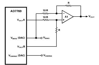
DAC A can be programmed to produce an interpolation function between the 8-bit steps of DAC B to allow, for example, very smooth velocity profile waveforms to be generated.
