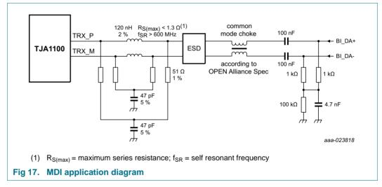
It is advised to use a PESD2ETH diode to protect against shorts to bus lines greater than 5 V. The supply terminal of the diode should be connected to a 3.3 V domain that is available when the TJA1100 is active. The diode layout should be symmetrical, as shown in the routing scheme example in Figure 18.
