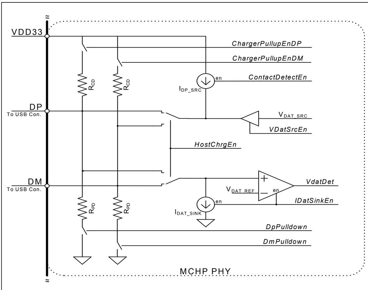
**Note:** The *italic names* in the [Figure 5-9](#) correspond to bits in the ULPI register set.
