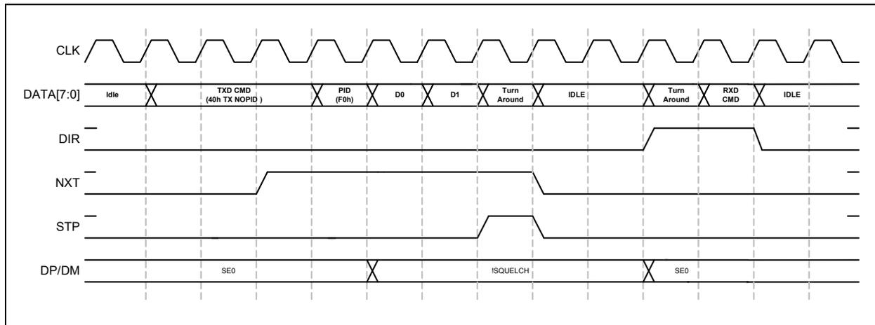
To send the 'F0' PID, the link will be required to use the TX CMD with NOPID to initiate the transmit and then follow up the TX CMD with the 'F0' PID. The data bytes follow as in a normal transmit, in *OpMode* 00b. The key difference is in that the link will have to send the PID the same as it would send a data packet. The USB334x is able to recognize the LPM transmit and correctly send the PID information.
