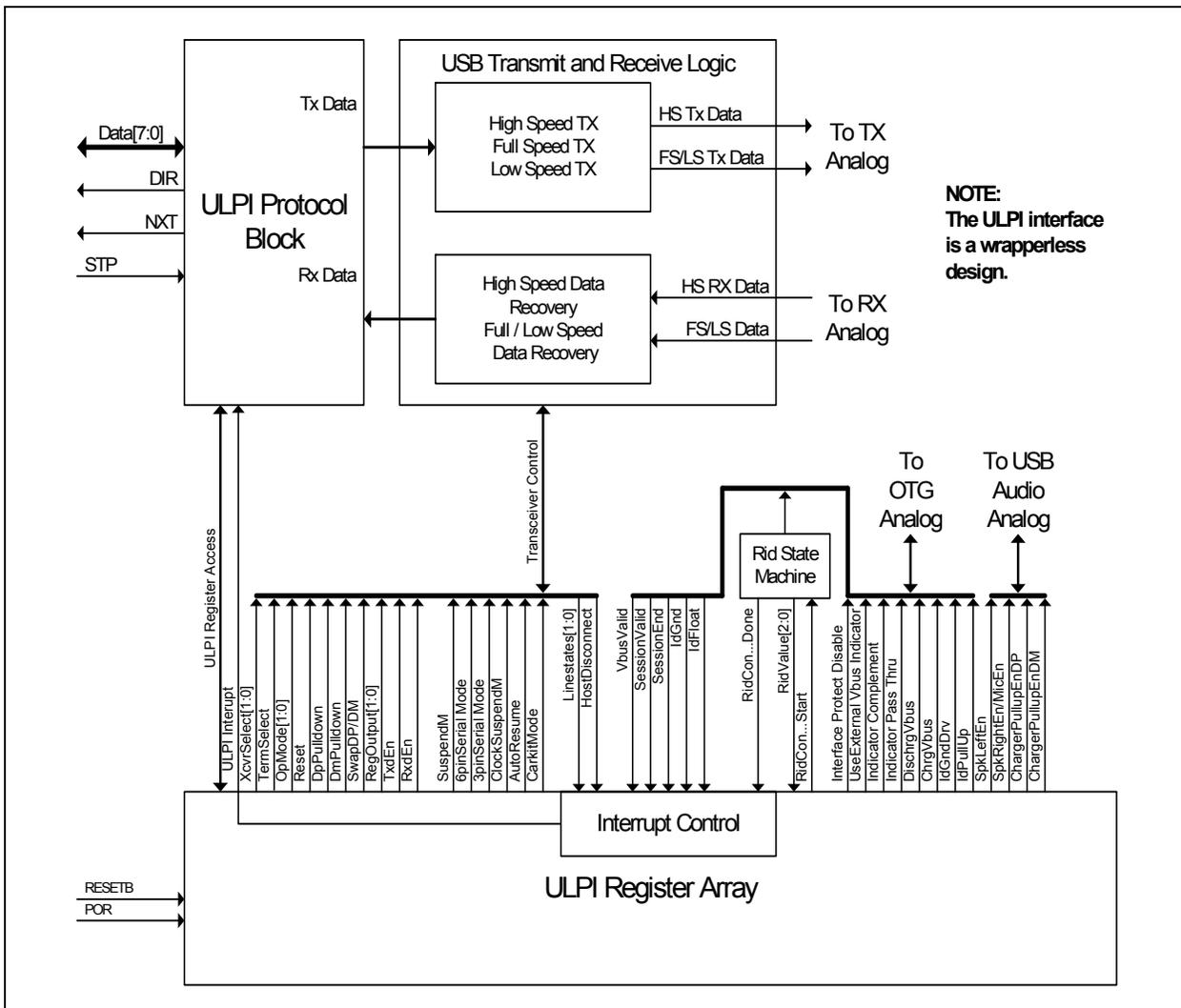
The advantage of a “wrapper-less” architecture is that the USB334x has a lower USB latency than a design which must first register signals into the PHY’s wrapper before the transfer to the transceiver core. A low latency PHY allows a wrapper around a UTMI Link to be used and still make the required USB turn-around timing required by the USB 2.0 specification.
