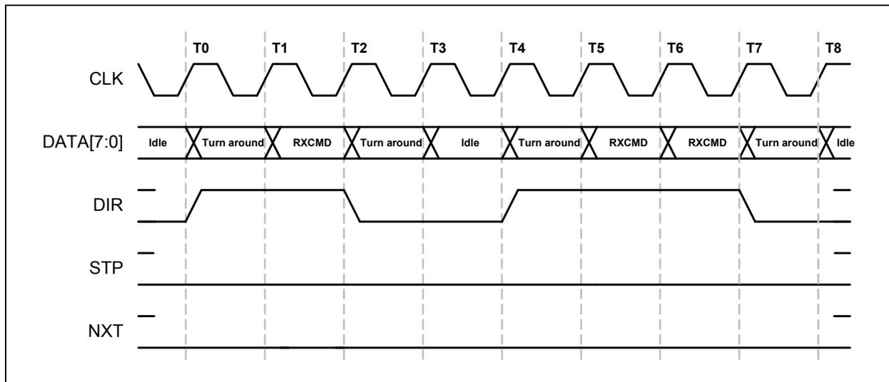
Transfer of the RXCMD byte occurs in Synchronous Mode when the PHY has control of the bus. The ULPI Protocol Block shown in [Figure 6-1](#) determines when to send an RXCMD. A RXCMD will occur:
