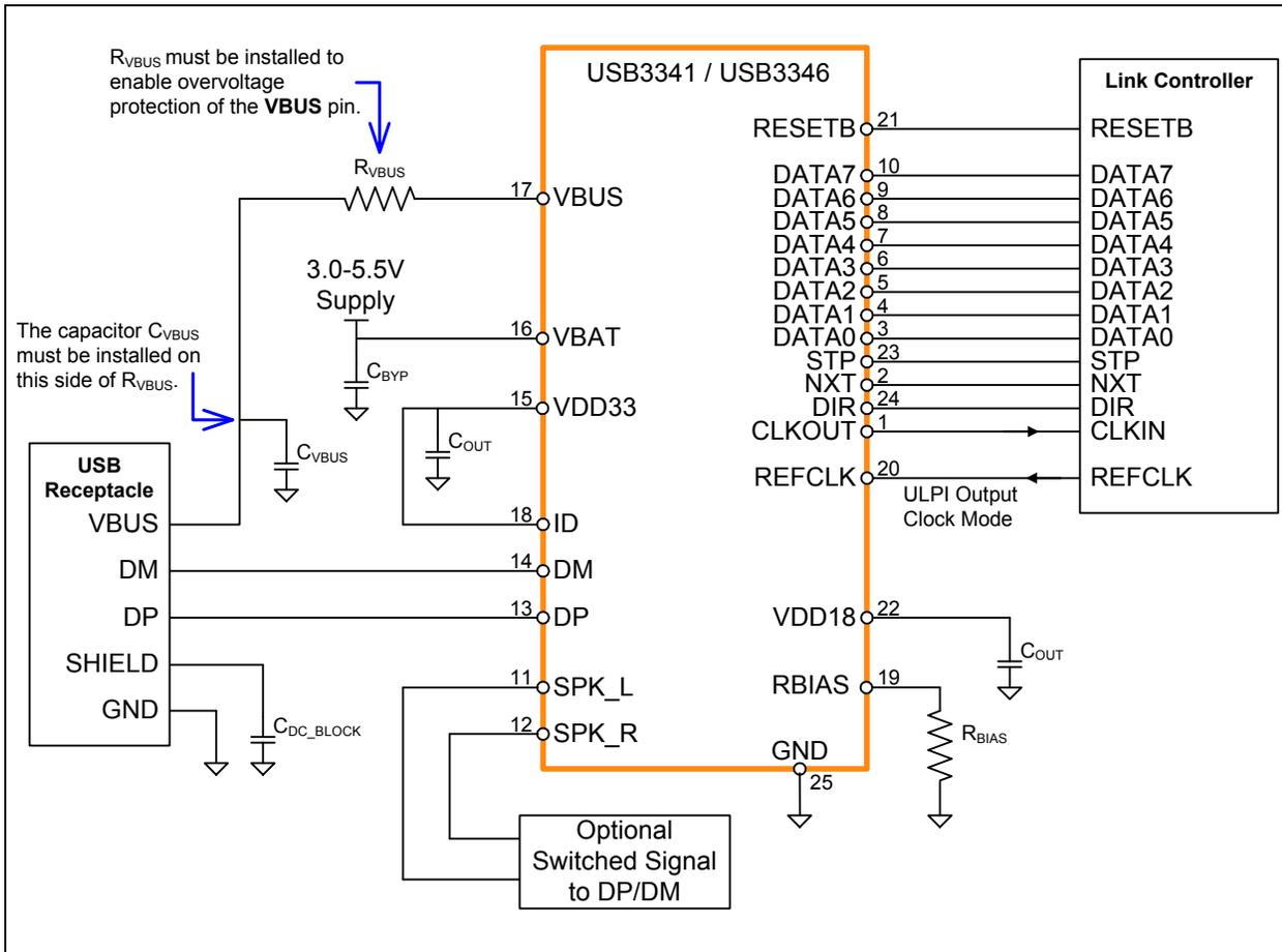
**FIGURE 8-2: USB3343 APPLICATION DIAGRAM (DEVICE CONFIGURED FOR ULPI CLOCK OUTPUT MODE)**
