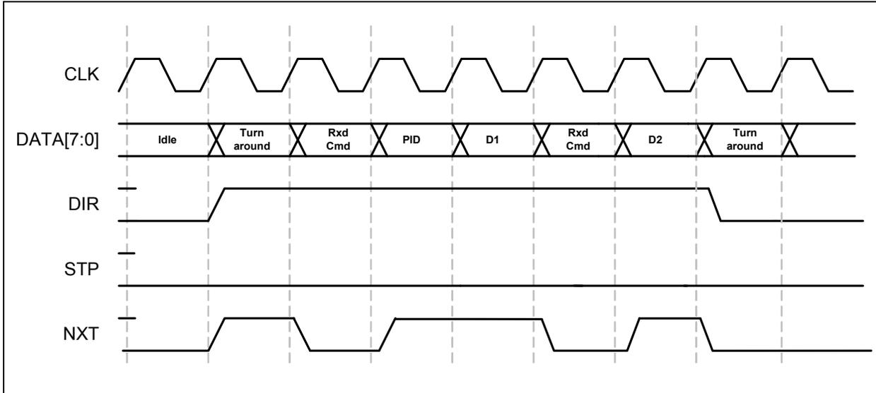
In [Figure 6-8](#) the PHY asserts **DIR** to take control of the data bus from the Link. The assertion of **DIR** and **NXT** in the same cycle contains additional information that Ractive has been asserted. When **NXT** is de-asserted and **DIR** is asserted, the RXCMD data is transferred to the Link. After the last byte of the USB receive packet is transferred to the PHY, the linestate will return to idle.
