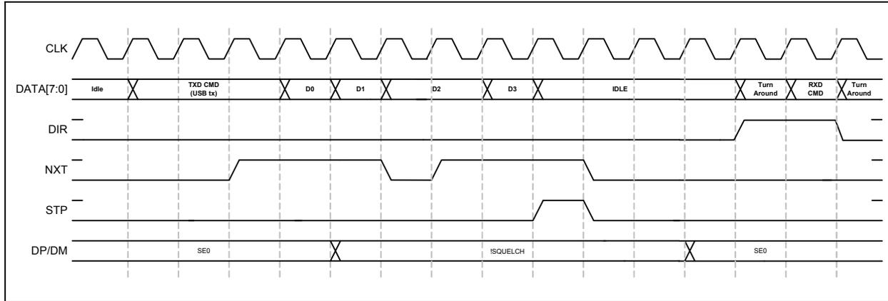
During transmit the PHY will use **NXT** to control the rate of data flow into the PHY. If the USB334x pipeline is full or bit-stuffing causes the data pipeline to overflow **NXT** is de-asserted and the Link will hold the value on Data until **NXT** is asserted. The USB Transmit ends when the Link asserts **STP** while **NXT** is asserted.
