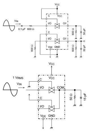
Figure 6 Cross Talk (between any two switches)
