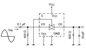
Figure 4 Feedthrough Attenuation
