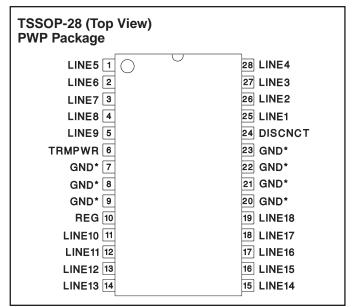
\* PWP package pin 23 serves as signal ground; pins 7, 8, 9, 20, 21, and 22 serve as heatsink ground.
