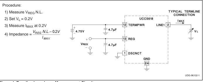
Figure 1. Termline Impedance Measurement Circuit
