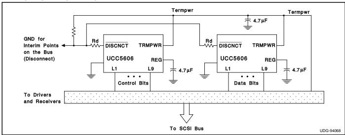
Figure 1: Typical SCSI Bus Configurations Utilizing 2 UCC5606 Devices
