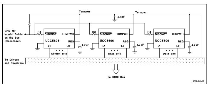
Figure 2: Typical Wide SCSI Bus Configurations Utilizing 3 UCC5606 Devices.
