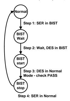
Figure 25. BIST Mode Flow Diagram
