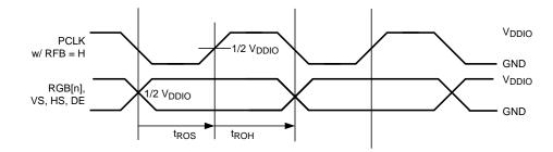
Figure 9. Deserializer Output Data Valid (Setup and Hold) Times with SSCG = Off
