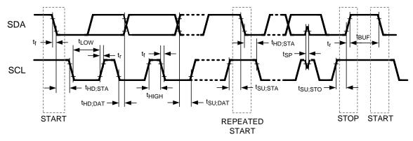
Figure 13. Serial Control Bus Timing Diagram
