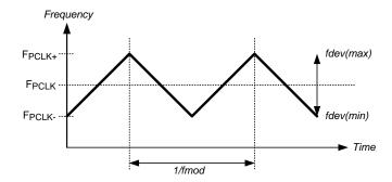
Figure 19. SSCG Waveform
