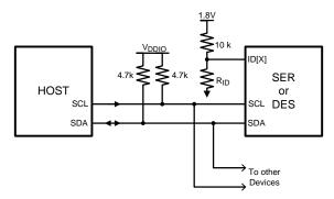
Figure 27. Serial Control Bus Connection
