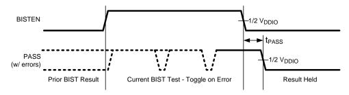
Figure 12. BIST PASS Waveform
