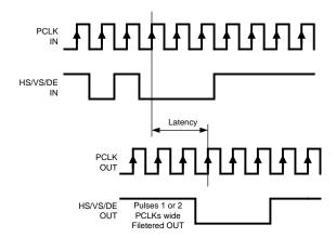
Figure 15. Video Control Signal Filter Waveform
