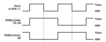
Figure 4. Checkerboard Data Pattern
