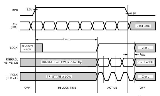
Figure 8. Deserializer PLL Lock Times and PDB TRI-STATE Delay<sup>(1)</sup>
