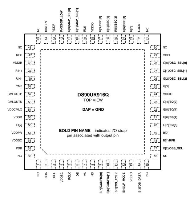
Figure 3. Deserializer - DS90UR916Q — Top View
