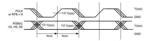
Figure 10. Deserializer Output Data Valid (Setup and Hold) Times with SSCG = On
