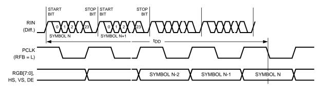
Figure 6. Deserializer Delay - Latency
