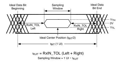
Figure 11. Receiver Input Jitter Tolerance
