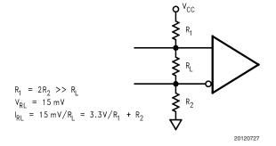
FIGURE 18. Failsafe Biasing Setup
