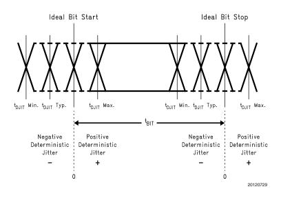
FIGURE 19. Deterministic Jitter and Ideal Bit Position
