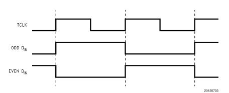
FIGURE 2. "Worst Case" Serializer ICC Test Pattern
