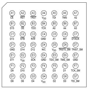
Figure 2. NFBGA Package Pinout (Top View)
