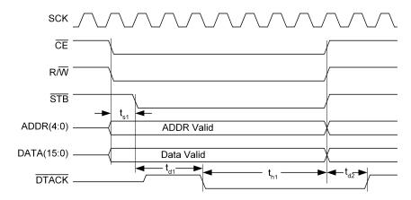
Figure 12. PPI Write Cycle Timing Diagram
