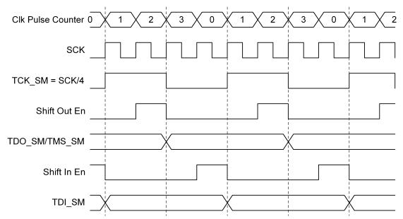
Figure 6. Shift Register Implementation and Timing
