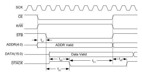
Figure 13. PPI Read Cycle Timing Diagram
