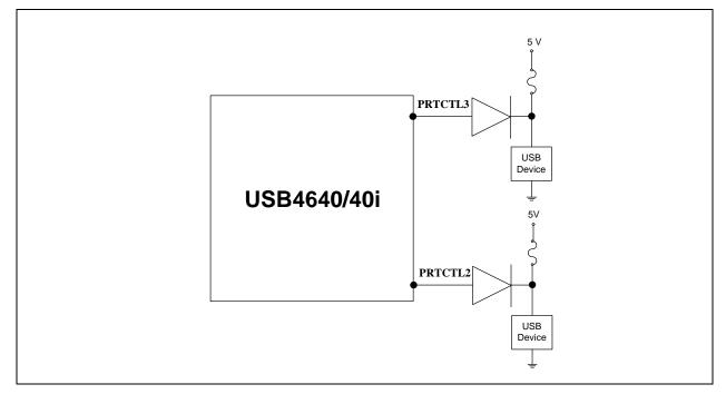
When using a single poly fuse to power all devices, note that for the ganged situation, all power control pins must be tied together.
