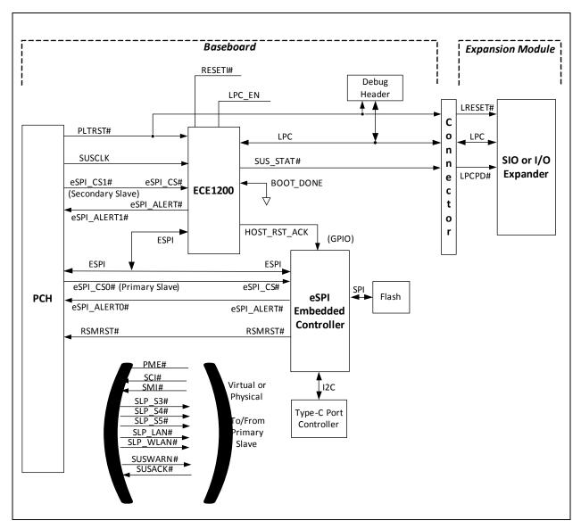
Note 1: This configuration has two eSPI Slaves. The ECE1200 is the Secondary slave device, with some limitations imposed by the Host PCH. It can receive any of the fixed Legacy decodes, but has only one Generic I/O decode range and one Generic Memory decode range available to it.
