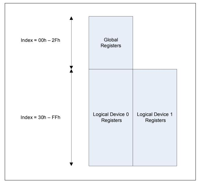
FIGURE 6-1: BLOCK DIAGRAM OF REGISTER SET
