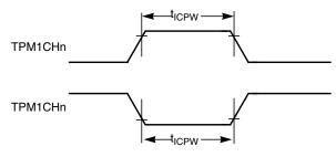
Figure A-10. Timer Input Capture Pulse
