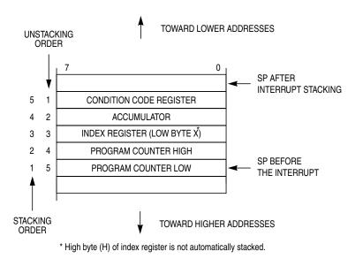
Figure 5-1. Interrupt Stack Frame
