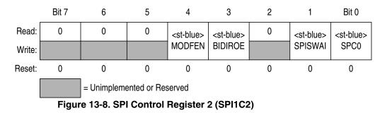
MODFEN — Master Mode-Fault Function Enable
