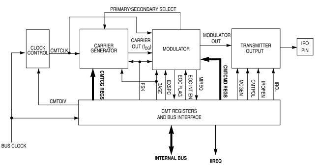
Figure 8-2. Carrier Modulator Transmitter Module Block Diagram
