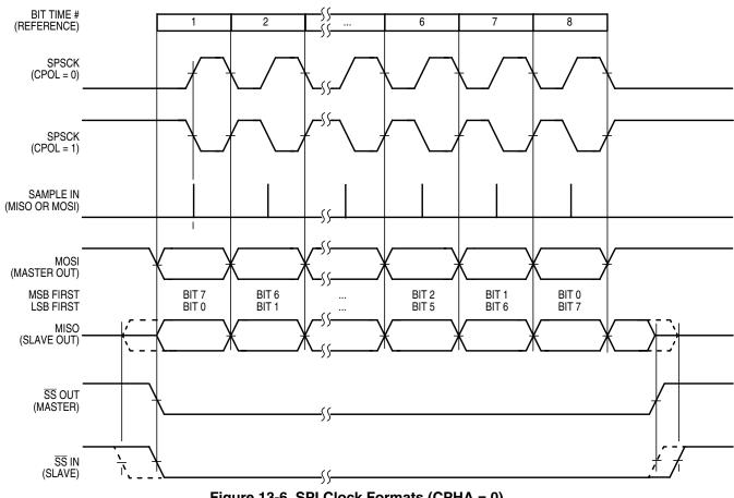
Figure 13-6. SPI Clock Formats (CPHA = 0)
