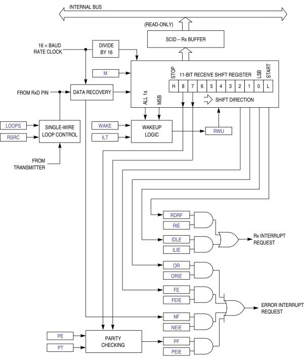
Figure 12-2. SCI Receiver Block Diagram
