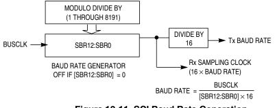
Figure 12-11. SCI Baud Rate Generation
