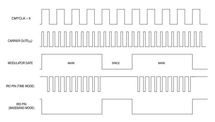
Figure 8-5. Example CMT Output in Time and Baseband Modes
