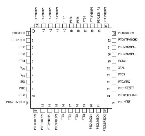
Figure 2-1. MC9S08RC/RD/RE/RG in 44-Pin LQFP Package
