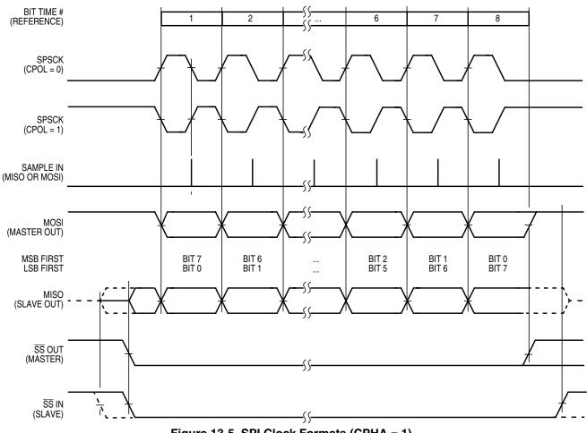
Figure 13-5. SPI Clock Formats (CPHA = 1)
