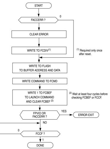
Figure 4-3. FLASH Program and Erase Flowchart
