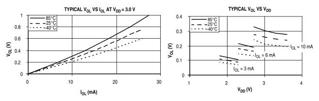
Figure A-2. Typical Low-Side Driver (Sink) Characteristics (Port B and IRO)
