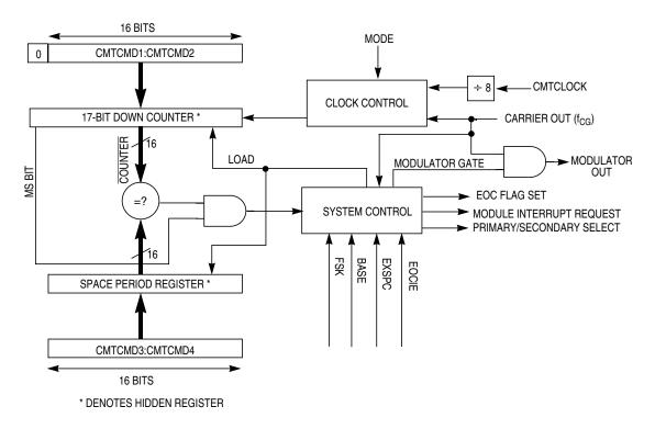
Figure 8-4. Modulator Block Diagram
