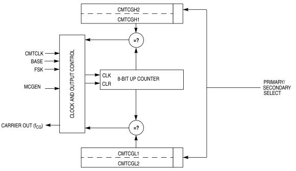
Figure 8-3. Carrier Generator Block Diagram
