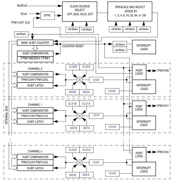
Figure 10-2. TPM Block Diagram
