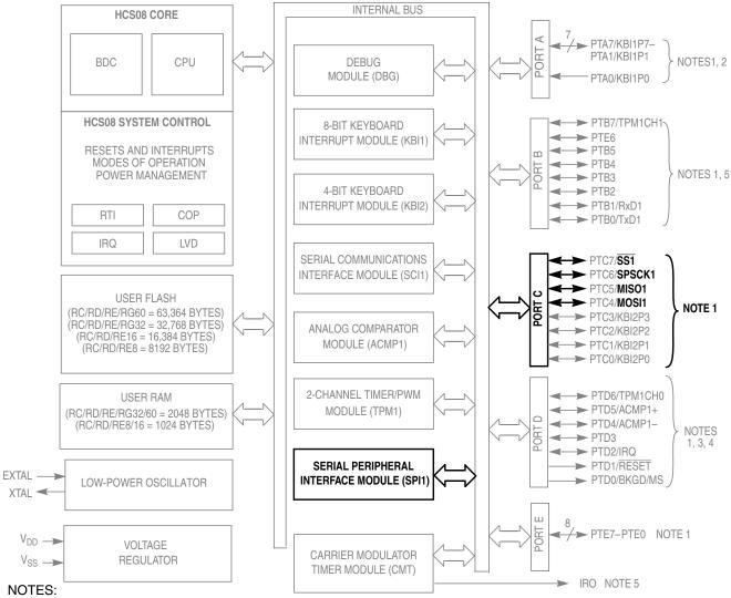
1. Port pins are software configurable with pullup device if input port
