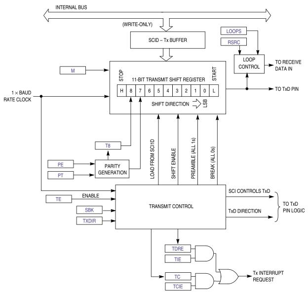
Figure 12-1. SCI Transmitter Block Diagram
