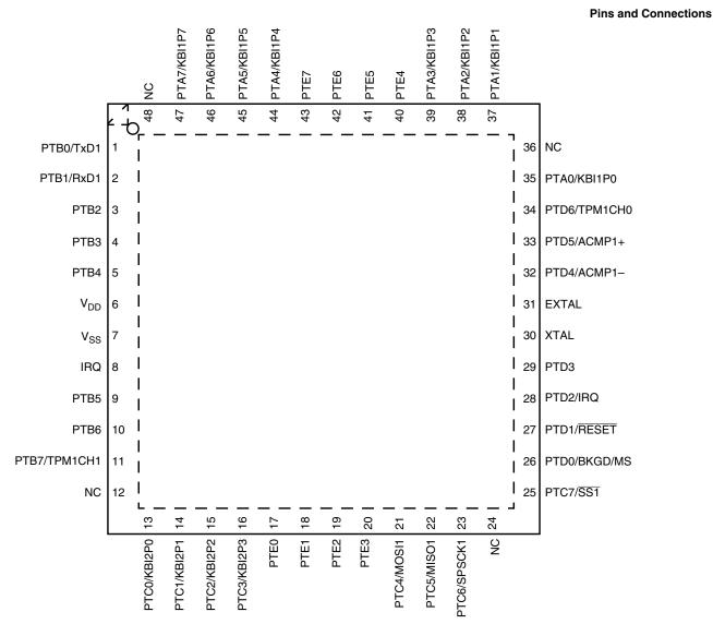
Figure 2-4. MC9S08RC/RD/RE/RG in 48-Pin QFN Package
