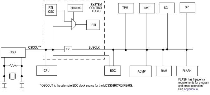
Figure 1-2. System Clock Distribution Diagram
