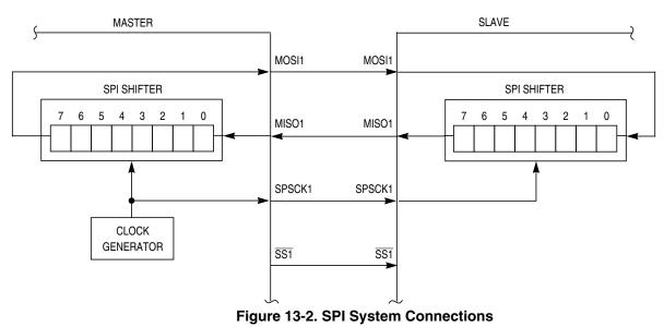
The most common uses of the SPI system include connecting simple shift registers for adding input or output ports or connecting small peripheral devices such as serial A/D or D/A converters. Although Figure 13-2 shows a system where data is exchanged between two MCUs, many practical systems involve simpler connections where data is unidirectionally transferred from the master MCU to a slave or from a slave to the master MCU.
