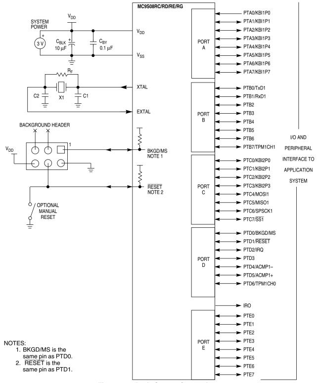
Figure 2-5. Basic System Connections
