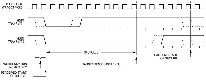
Figure 15-2. BDC Host-to-Target Serial Bit Timing
