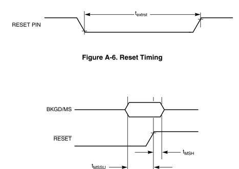
Figure A-7. Active Background Debug Mode Latch Timing
