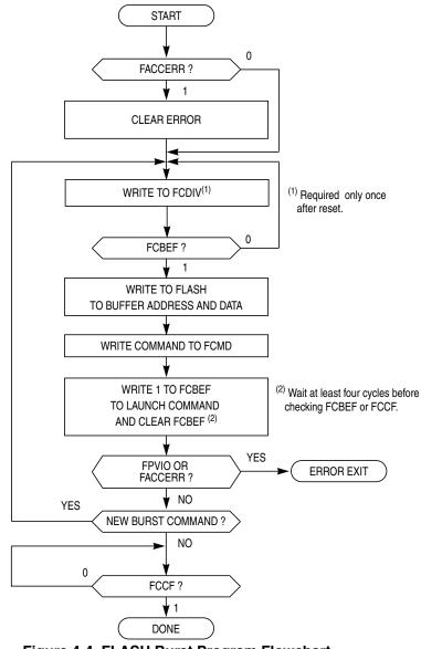
Figure 4-4. FLASH Burst Program Flowchart
