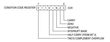
Figure 7-2. Condition Code Register
