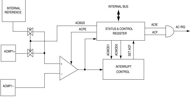
Figure 14-2. Analog Comparator Module Block Diagram
