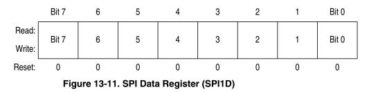
Reads of this register return the data read from the receive data buffer. Writes to this register write data to the transmit data buffer. When the SPI is configured as a master, writing data to the transmit data buffer initiates an SPI transfer.
