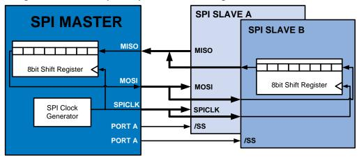
In Figure 7-5, slave's SSIG = 0, and SS is used to select the slave. The SPI0 master can use any port pin (including P5.0/SS with SSIG = 1) to drive the SS pin.
