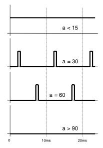
**In case that PWM mode is selected**, these four registers are used to adjust the duty cycle. In this case, each one must contain a value between 0 and 255 (0xFF). When 255 (0xFF), PWM output is always VDD.
