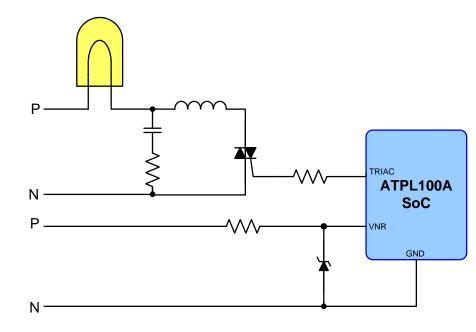
Figure 9-6. Phase Control with "non-isolated connection"
