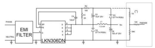
"This Resistor must support high voltages
