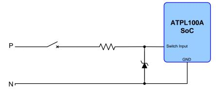
Figure 9-10 shows how to connect a low voltage switch to the integrated circuit.
