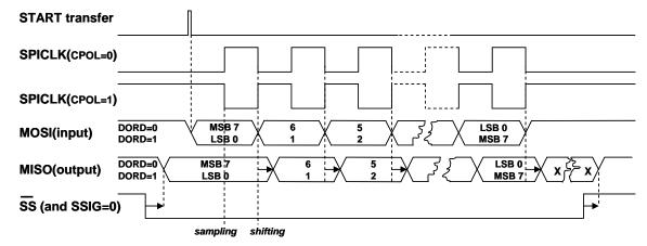
Figure 7-3. SPI0 transfer with CPHA=1
