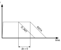
Not minimum time is required between both releases,  $\Delta t > 0$ , so a simple RC circuit is enough to satisfy this requirement.
