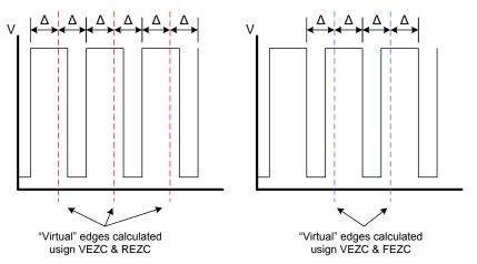
VECZ can be used simultaneously with REZC or FECZ.
