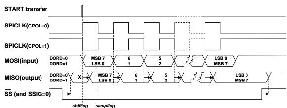
Note that the master selects a slave by driving the slave select pin of the corresponding slave device. Data written to the SPDAT register of the master is shifted out of the MOSI pin of the master to the MOSI pin of the slave, at the same time the data in SPDAT register on slave side is shifted out on its MISO pin to the MISO pin of the master.
