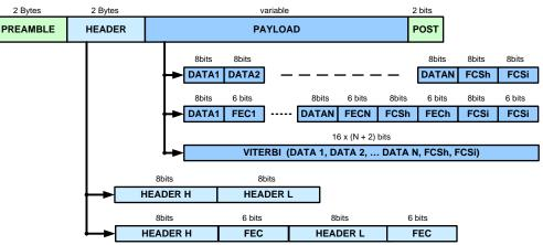
A standard packet encapsulation has the following structure
