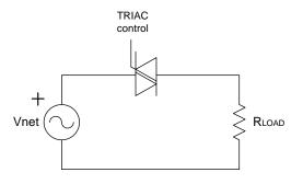
The firing angle ( $\alpha$ ) of the switch can be varied. The average voltage will be proportional to the area under the sine wave. Thus, the average voltage is the integral from the firing angle to the zero crossing.
