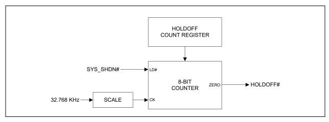
The SCALE function reduces the 32.768KHz clock to 8Hz, so that the 8-bit counter counts intervals of 125ms. The following table shows some of examples of the effect of several settings of the Holdoff Count Register:
