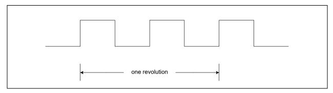
In typical systems, the fans are powered by the main power supply. Firmware may disable this block when it detects that the main power rail has been turned off by either clearing the <enable> TACH\_ENABLE bit or putting the block to sleep via the supported Low Power Mode interface (see Low Power Modes).
