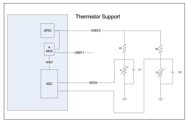
FIGURE 21-3: ADC REFERENCE VOLTAGE CONNECTION
