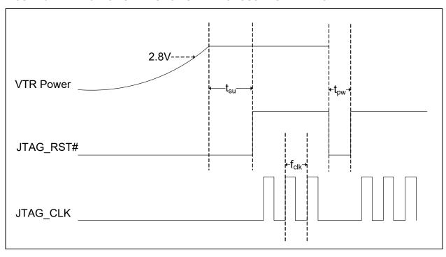
FIGURE 34-13: JTAG SETUP & HOLD PARAMETERS
