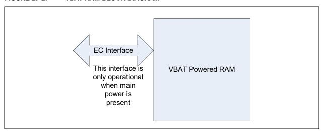
The VBAT Powered RAM provides a 64 Byte Random Accessed Memory that is operational while VTR\_CORE is powered, and will retain its values powered by VBAT while VTR\_CORE is unpowered. The RAM is organized as a 16 words x 32-bit wide for a total of 64 bytes.
