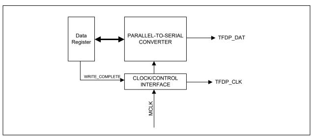
The firmware executing on the embedded controller writes to the Debug Data Register to initiate a transfer cycle (Figure 25-2). The Debug Data Register is loaded into a shift register and shifted out on TFDP\_DAT LSB first at the programmed TFDP\_CLK Clock rate (Figure 25-3).
