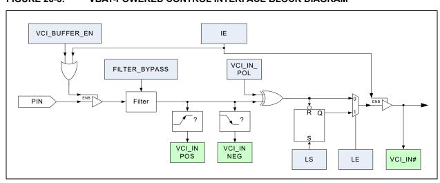
FIGURE 26-3: VBAT-POWERED CONTROL INTERFACE BLOCK DIAGRAM
