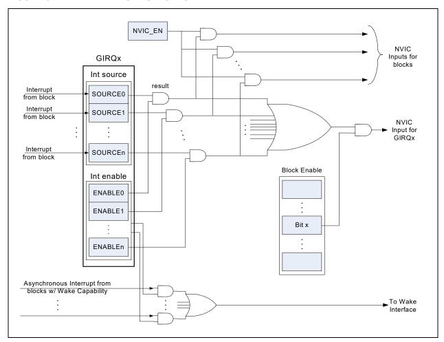
FIGURE 8-2: INTERRUPT STRUCTURE
