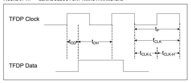
TABLE 34-11: SERIAL DEBUG PORT INTERFACE TIMING PARAMETERS
