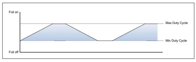
The clipping periods at the two extremes can be adjusted independently, so that for example an LED can appear to breathe (with a short delay at maximum brightness) followed by a longer "resting" period (with a long delay at minimum brightness).
