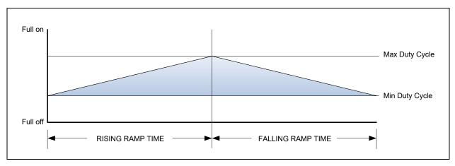
The breathing range of and LED can range between full on and full off, or in a range that falls within the full-on/full-off range, as shown in this figure. The ramp time can be different in different applications. For example, if the ramp time was 1 second, the LED would appear to breathe quickly. A time of 2 seconds would make the LED appear to breathe more leisurely.
