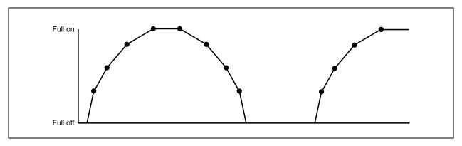
In this figure, the rise and fall curves are implemented in 4 linear segments and are the rise and fall periods are symmetric.
