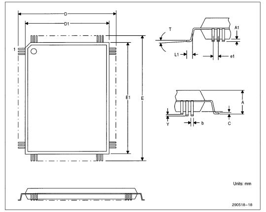
Figure 16. 100 Pin Plastic Quad Flat Pack (PQFP) Dimensions
