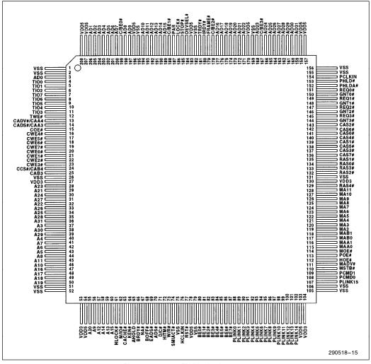
Figure 13. 82437FX Pin Assignment
