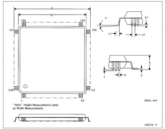
Figure 15. 208 Pin Quad Flat Pack (QFP) Dimensions
