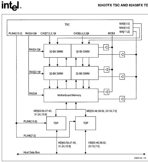
Figure 8. DRAM Array Connections
