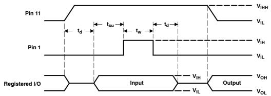
NOTE 3:  $t_d = t_{su} = t_h = 100 \text{ ns to } 1000 \text{ ns } V_{IHH} = 10.25 \text{ V to } 10.75 \text{ V}$
