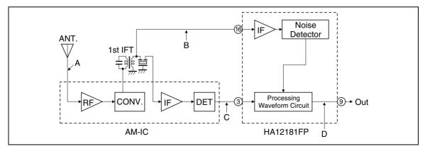
Figure 2 System Block Diagram of AM Radio
