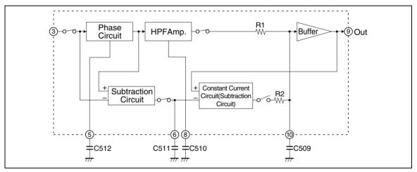
Figure 4 Waveform Processing Circuit
