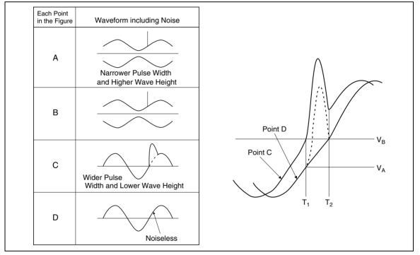
Figure 3 Waveforms at Each Point in the System
