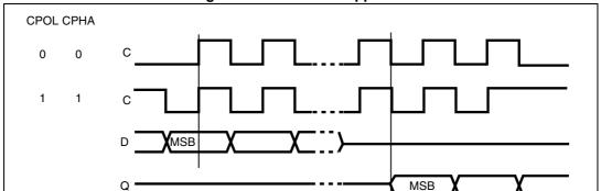
Figure 6. SPI modes supported
