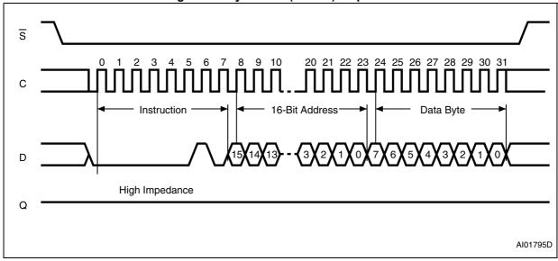
Figure 13. Byte Write (WRITE) sequence
