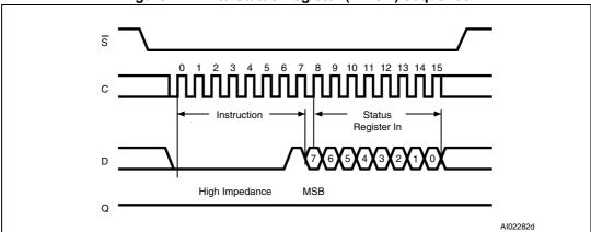
Figure 11. Write Status Register (WRSR) sequence
