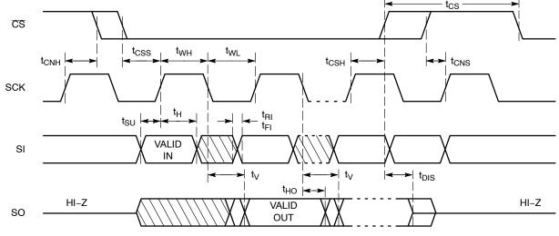
Figure 2. Synchronous Data Timing
