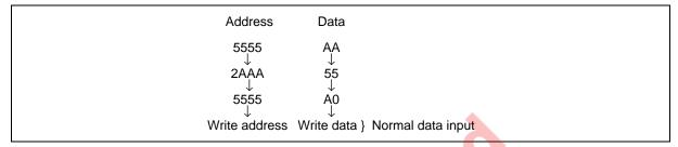
The SDP mode is disabled by inputting the following 6 bytes code. Note that, if data is input in the SDP disable cycle, data can not be written.
