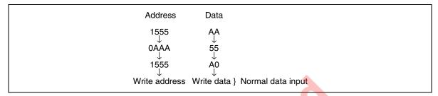
Software data protection mode can be canceled by inputting the following 6 bytes. After that, this device turns to the non-protection mode and can write data normally. But when the data is input in the canceling cycle, the data cannot be written.
