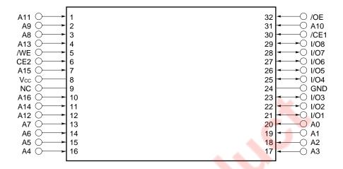
A0 - A16 : Address inputs /OE : Output Enable I/O1 - I/O8: Data inputs / outputs Vcc : Power supply
