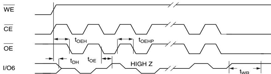
Notes: 1. Toggling either  $\bar{O}\bar{E}$  or  $\bar{C}\bar{E}$  or both  $\bar{O}\bar{E}$  and  $\bar{C}\bar{E}$  will operate toggle bit. The  $t_{OEHP}$  specification must be met by the toggling input(s).
