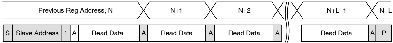
Figure 21. Sequential READ, Start from Current Location
